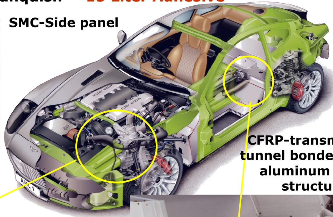
CFRP-transmission tunnel bonded to the aluminum body structure
